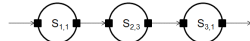
Fig. 7. Internal reconfiguration; taking figure 5 as starting point, the application replaces s_{2,2} of figure 5 by a companion
